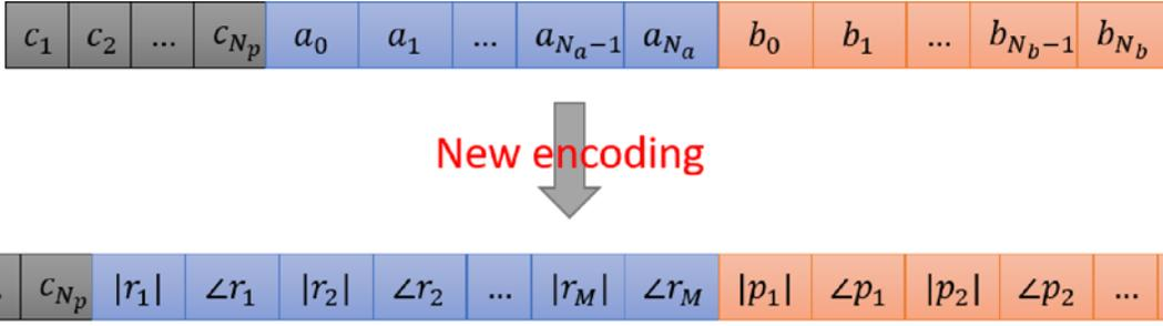
Fig. 2: New proposal of parameter vector of each CLONALG individual, in comparison to the former approach.
