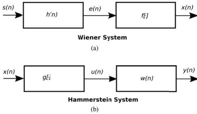
Fig. 1: Diagram of Wiener and Hammerstein systems.
